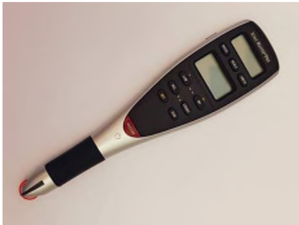
Figure 3.11 – A digital measuring wheel (Scale Master Pro) for measuring the crack length.
