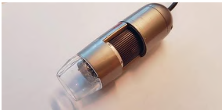
Figure 3.9 – The Dino Lite AM-413T Pro digital microscope, used for measuring the crack width.
