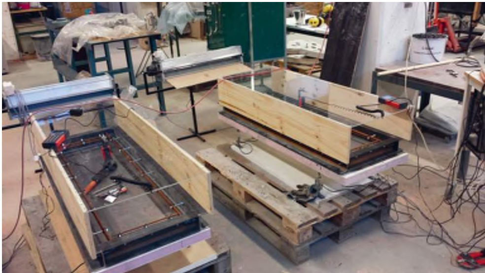
Figure 3.5 – Two rectangular mould test setups with fans and wind tunnels, placed on four load-cells.
