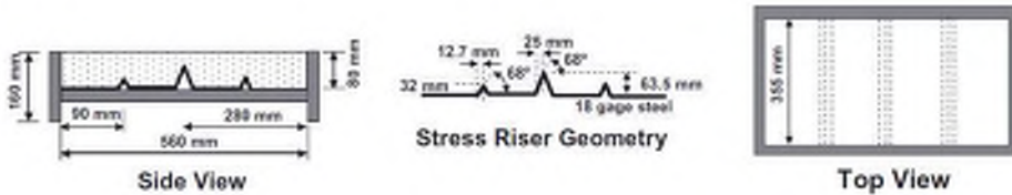
Figure 2: Restrained shrinkage test setup, manufactured according to ASTM C 1579 [34], figure based on [35].
