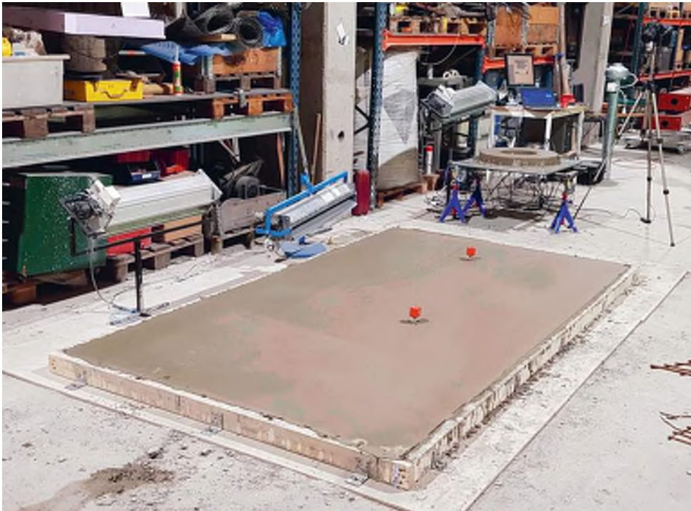
Figure 3.15 – The half-scale test setup, including the slab and the ring test mould, after casting.
