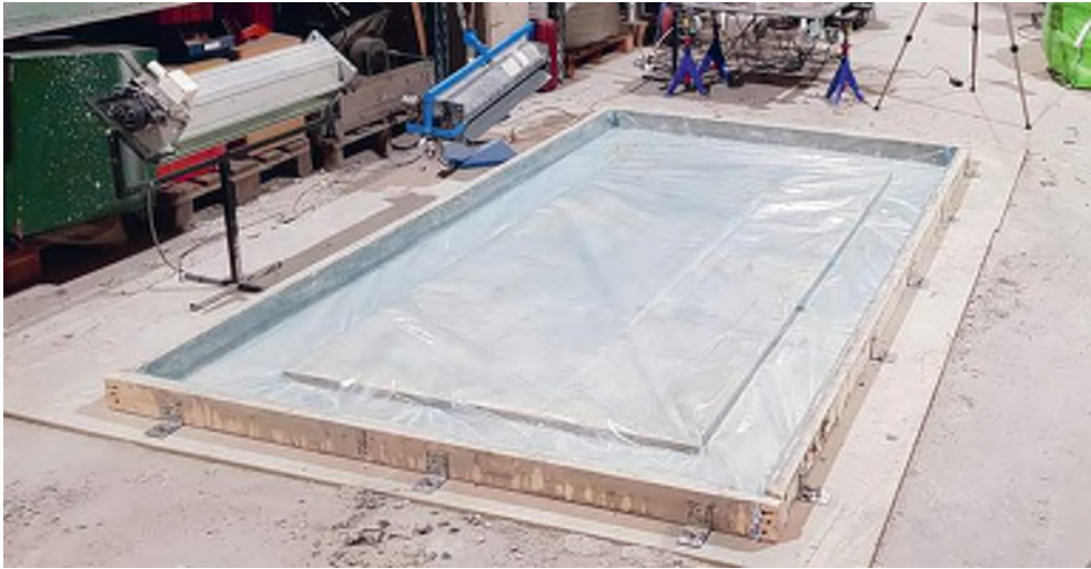
Figure 3.14 – The half-scale mould before casting.
