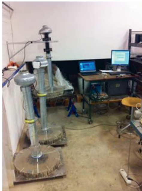
Figure 3.4 - Arrangement of the three moulds in the ring test method.
